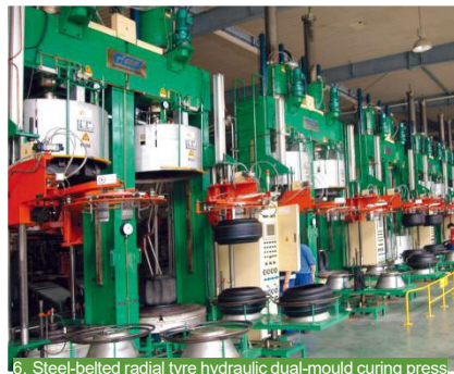
6. Steel-belted radial tyre hydraulic dual-mould curing press
