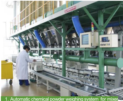
1. Automatic chemical powder weighing system for mixer
